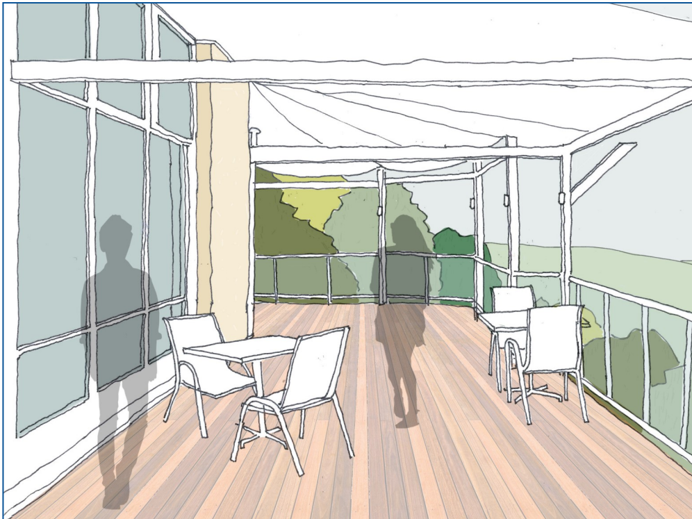
New Spotted Gum decking with new balustrades
